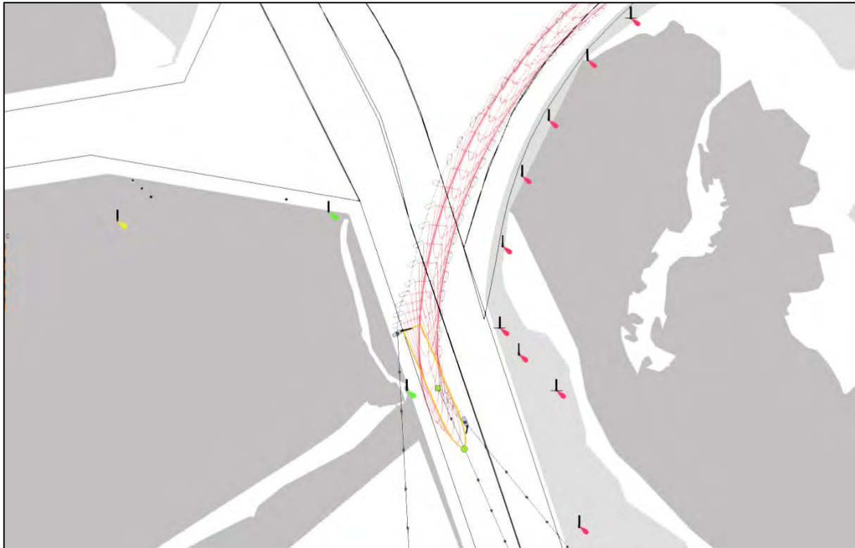
Screenshot 11E. Ship Turning into HSC at 8kn scraping along the bottom of the HSC
