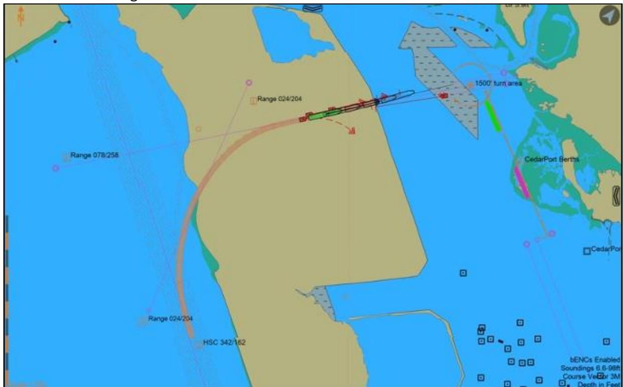
Screenshot 41B. Ship after performing arcing turn onto second set of ranges at 078° headed into turning basin
