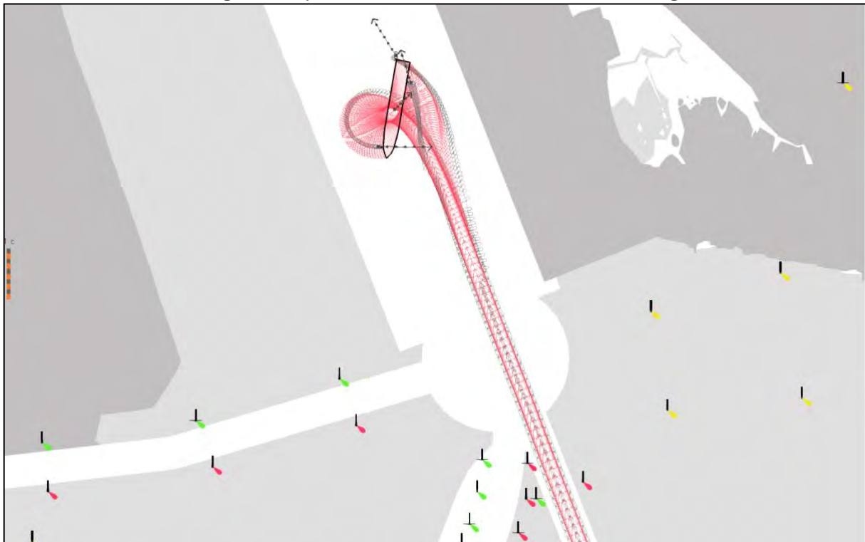
Screenshot 1G. Turning the Ship in the Terminal Basin After Transiting Channel Delta
