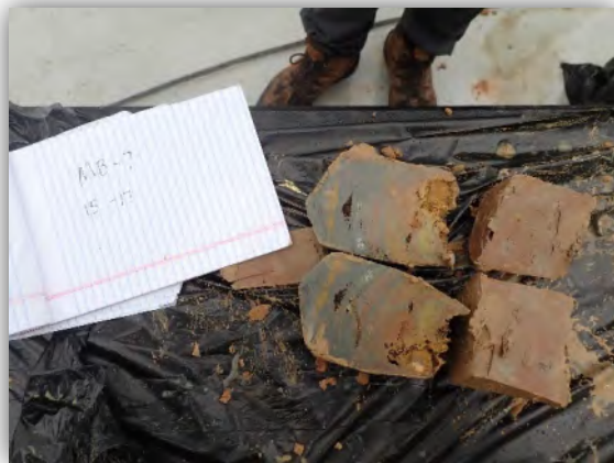
5. Marine Core MB-7 at the 15-17 Foot Interval Sliced & Splayed
