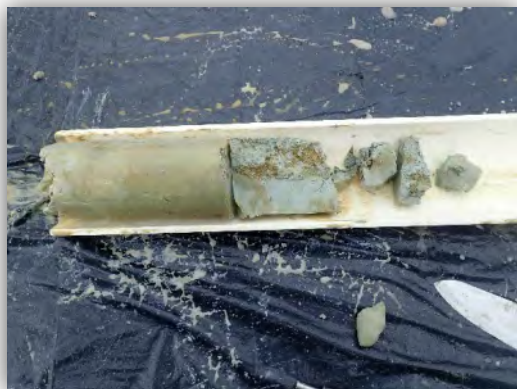
7. Typical High-Clay Portion of a Full-Depth Core Interval for Observation/Description
