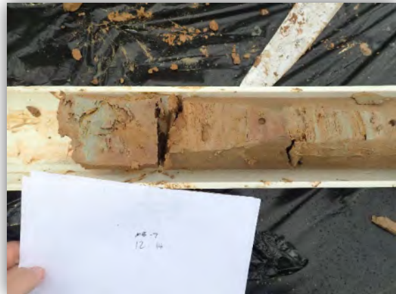
4. Example of Brown and Gray Clays Encountered in Full-Depth Cores.
