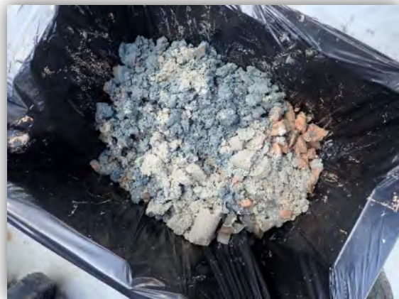
6. Typical Full-Depth Core Broken into Lined Container for Forming Composite
